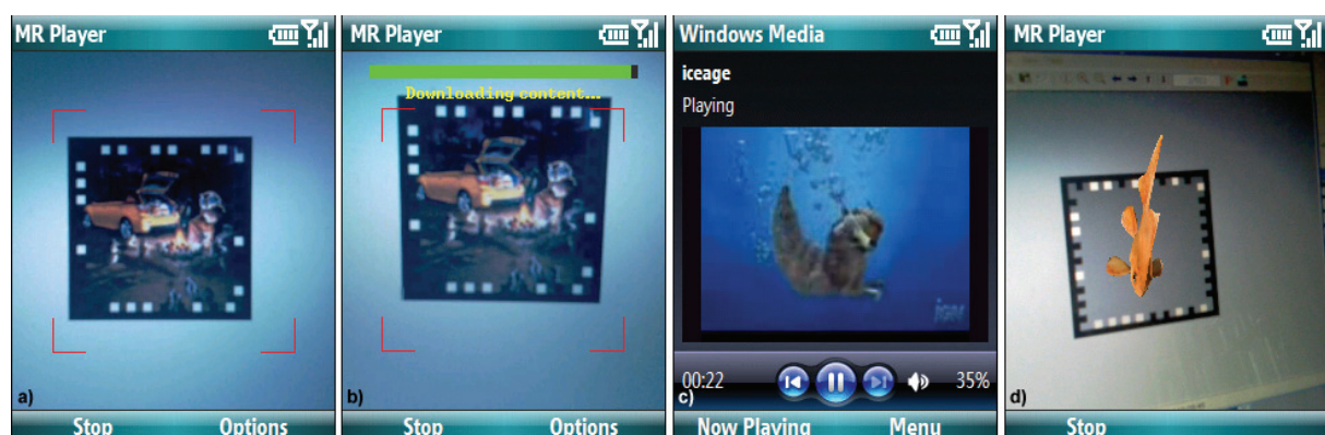
Figure 14: Screenshots of the MR-Player application in use: a) User points the camera at a visual marker. b) Content is downloaded from the server. c) Video playback. d) 3D geometry presented overlaid onto the marker.
